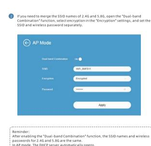
After enabling the "Dual-band Combination" function, the SSID names and wireless passwords for 2.4G and 5.8G are the same. In AP mode, The DHCP server automatically opens.
